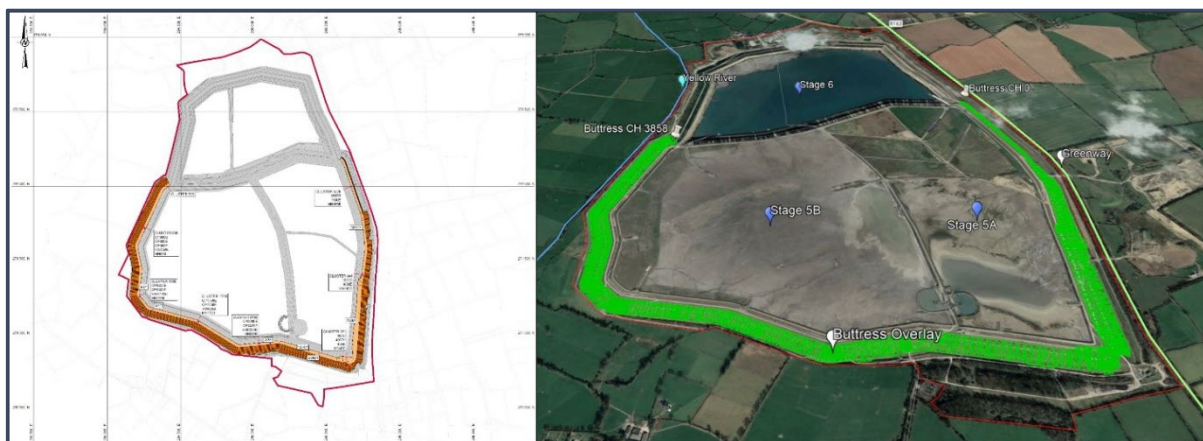
Figure 3.5 Tailings Facility and Proposed Buttress Layout Plan
